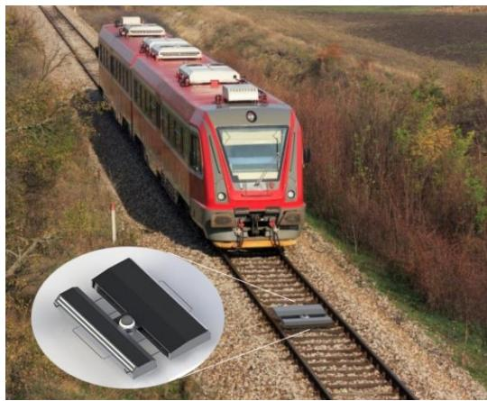
**ATUVIS : FME researchers are developing Autonomous robot for train undercarriage visual inspection**
