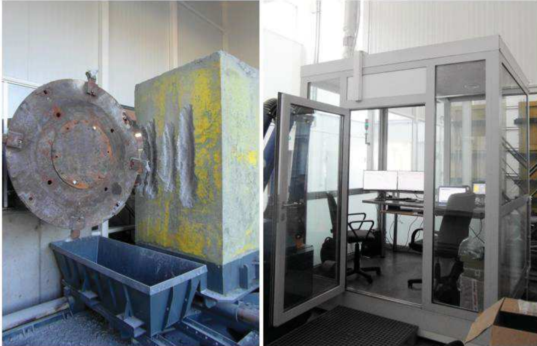
Fig. 2. Laboratory test stand to research cutting process or rotation drilling with use of single cutting tool or cutting head
