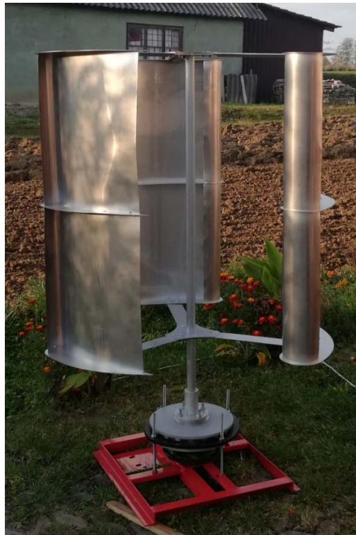
Fig.2. Power station with a vertical axis of rotation
