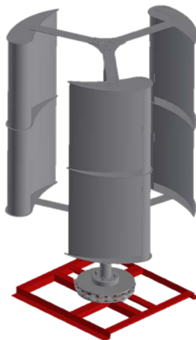
Fig.1. Assembly model of a power plant with a vertical axis of rotation
