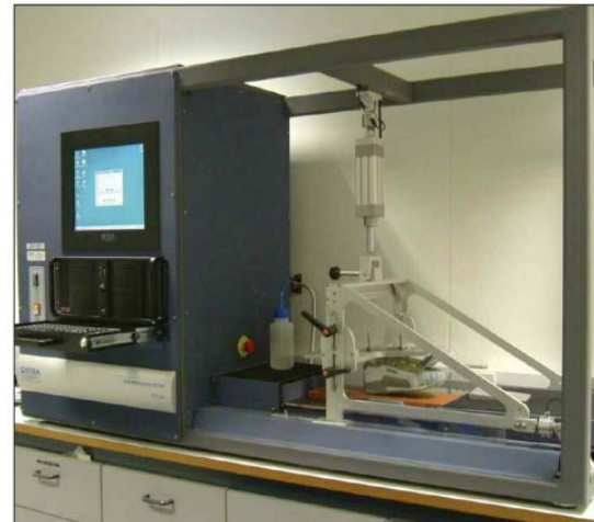
Fig. 3. Test equipment for measurement the slip resistance of footwear [15]
