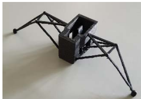
Fig. 4 Prototype of the terrestrial walking soft robot design 1 realized with 3D printing
