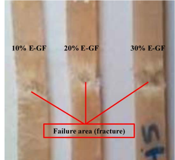
Fig 7. images of a sample of the content of glass fiber, 10%, 20% and 30% when reaching the fatigue limit.
